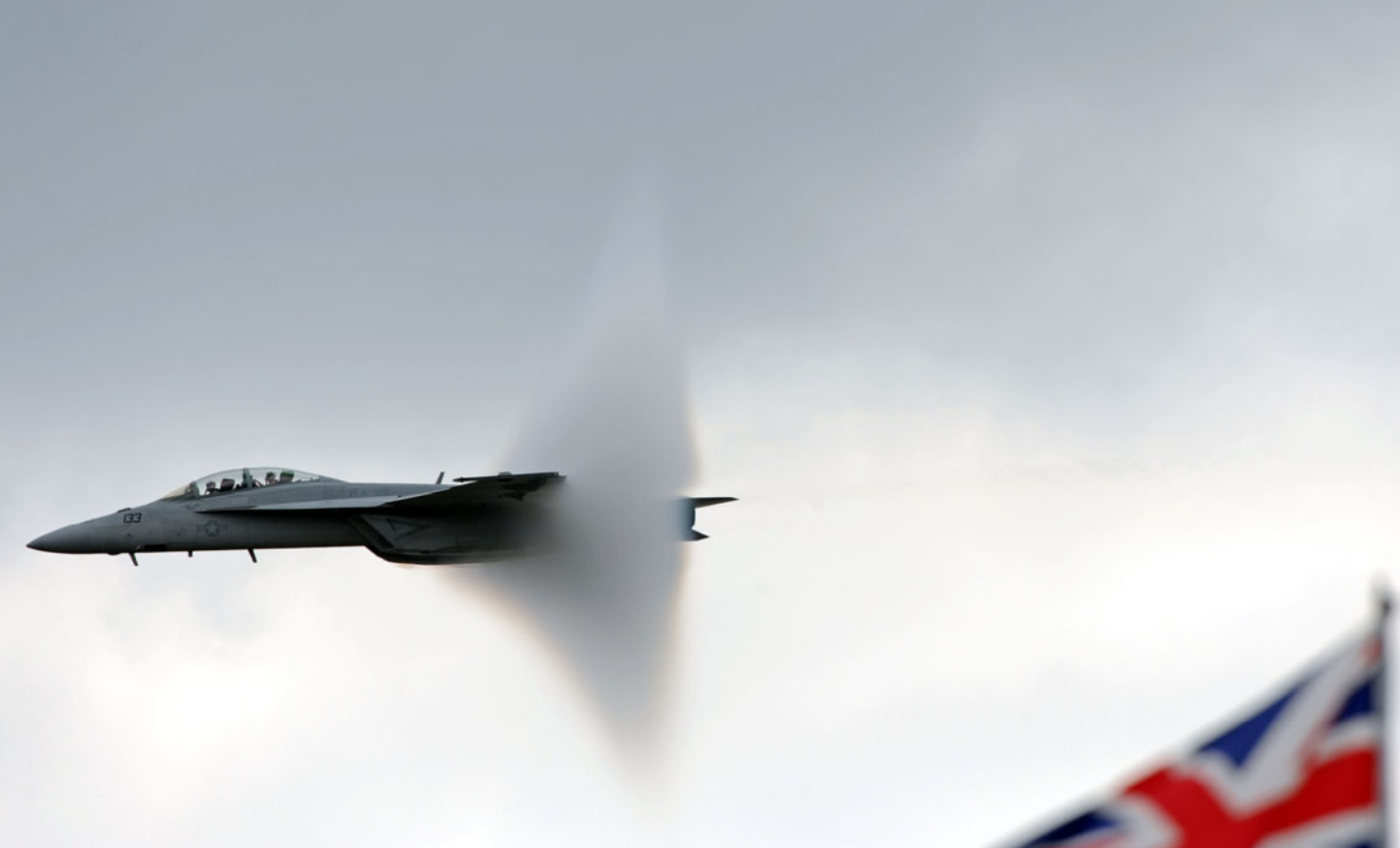
F/A-18F Super Hornet "Rhino" with vapour cone, flying close to the speed of sound, at the Abbotsford Air
