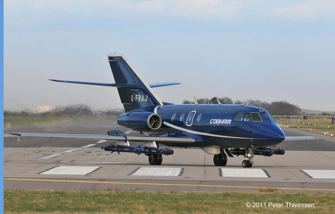
Dassault Falcon 20 FRADU (Fleet Requirements and Air Direction Unit) aircraft from Bournemouth, providing ECM and radar threat simulation .
