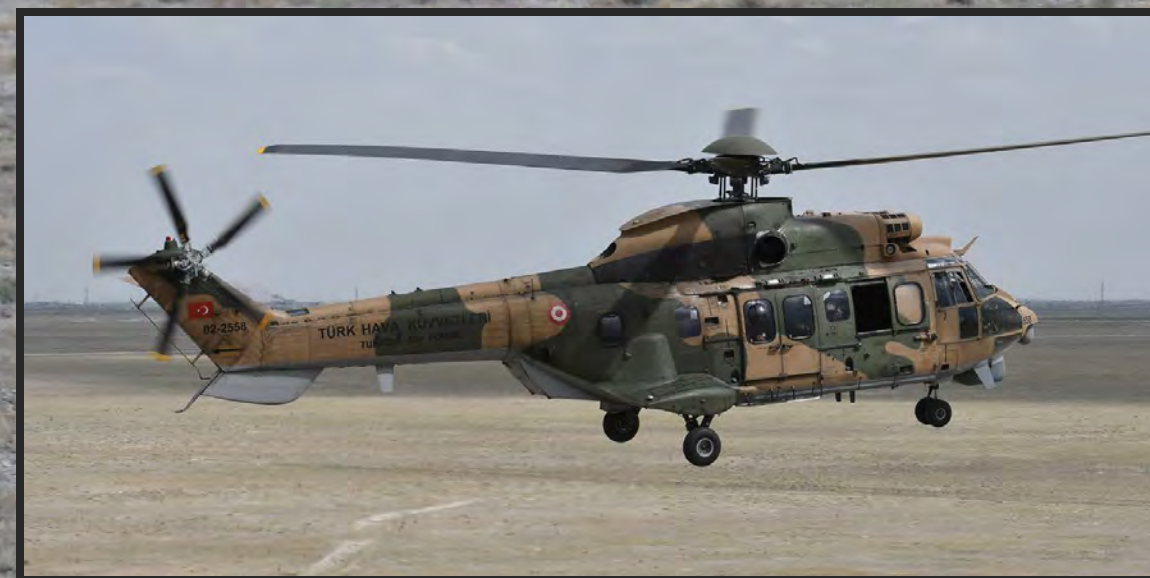
Turkish Air Force AS532UL Cougar assigned to 135 Filo. The door-gunner with his machine gun is tasked with the suppression of hostile action on the ground against the helicopter approaching the landing zone to deploy extraction forces. This CSAR configured Cougar also carries a gunpod attached to the left side of the fuselage ( main image and left inset ).
