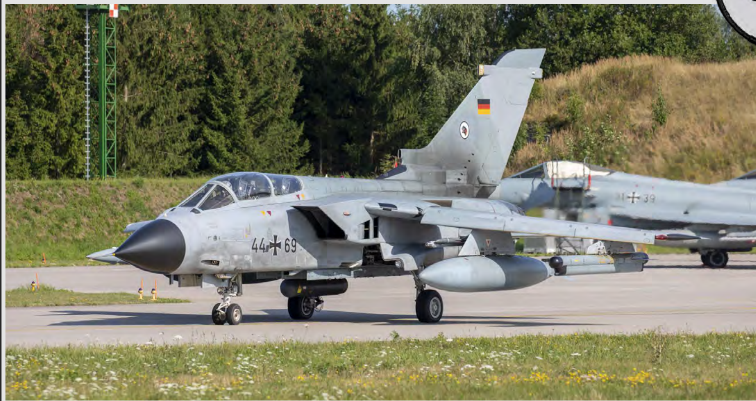
Tornado IDS (left) and Tornado ECR (right) configured with a LITENING target designating pod on the underfuselage pylon, two 410 gal (1,552 l) external fuel tanks on the inner wing pylon, an IRIS-T air-to-air missile on the left wing's inner pylon, a chaff and flare dispenser on the outer pylon of the right wing, and the TSPJ (Tornado Self Protection Jammer) ECM pod on the left wing's outer pylon.
