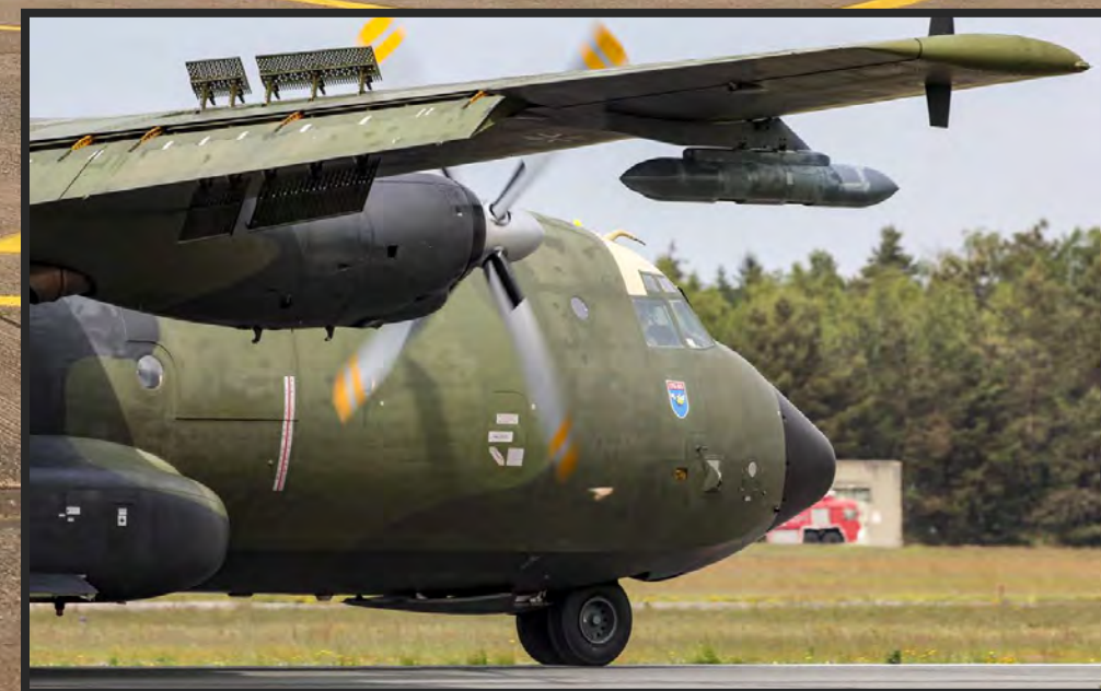
Speedbrakes on the upper and lower wing surface and the flaps fully deployed indicate that this Transall just had landed
