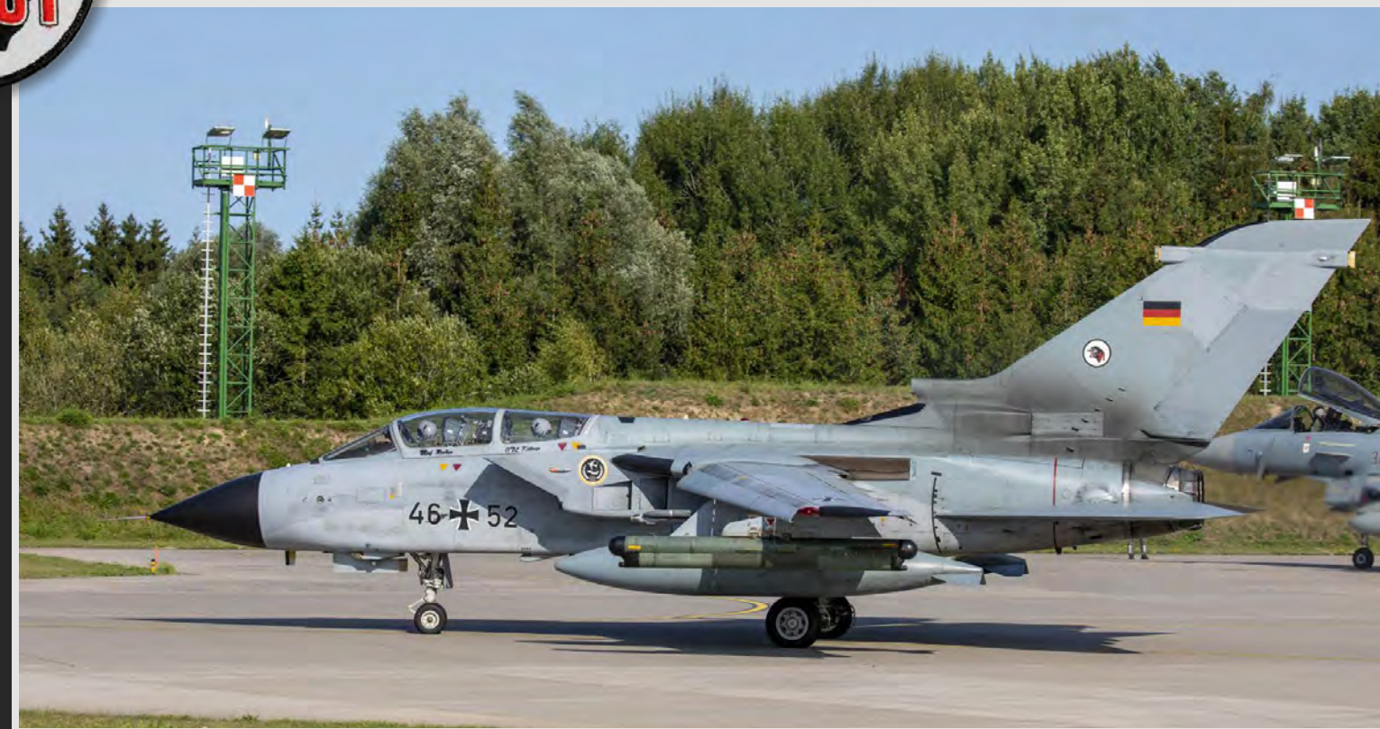
Tornado IDS (left) and Tornado ECR (right) configured with a LITENING target designating pod on the underfuselage pylon, two 410 gal (1,552 l) external fuel tanks on the inner wing pylon, an IRIS-T air-to-air missile on the left wing's inner pylon, a chaff and flare dispenser on the outer pylon of the right wing, and the TSPJ (Tornado Self Protection Jammer) ECM pod on the left wing's outer pylon.
