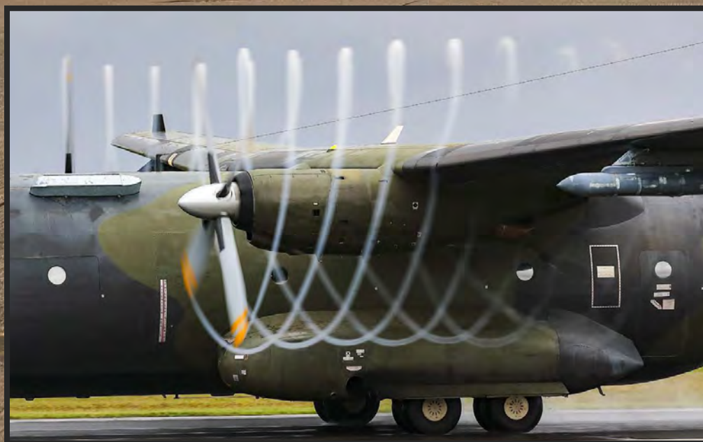
Due to the low pressure created at the propeller blade tips at high speeds and high humidity, the moisture condenses making the tip vortices visible.
