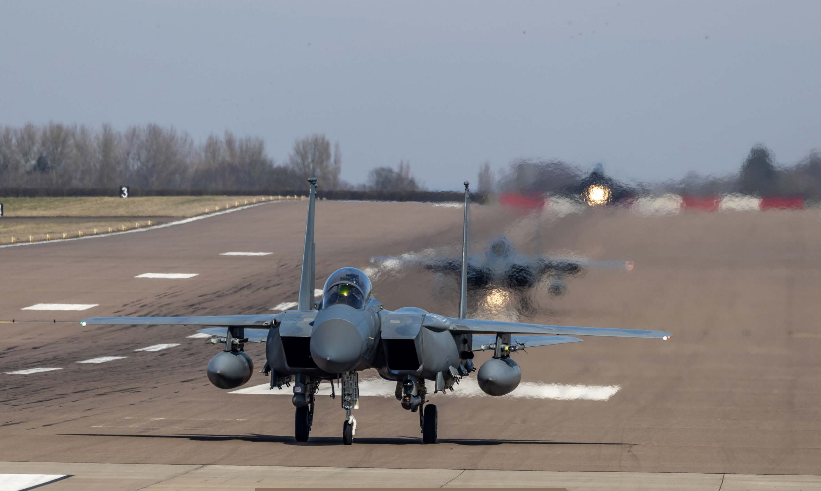
For air combat, the F-15SA carries an AIM-9X Sidewinder short-range air-to-air missile, an AN/AAQ-33 SNIPER targeting pod on the left fuselage station, and an AN/AAQ-13 LANTIRN navigation pod on the right. The navigation pod contains a terrain-following radar and an infrared detector. This enables the aircraft to maintain a predetermined altitude above ground and to avoid obstacles
