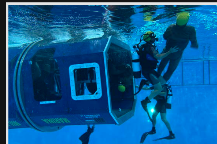
The modular egress training system ("Helo Dunker") can simulate a forced landing of a helicopter in the water and is used to train crews to escape safely from an underwater, upside down position. This requires also the removal of one of the helicopter's doors. Not an easy task that everyone has to pass every year to be qualified to operate in a Navy helicopter
