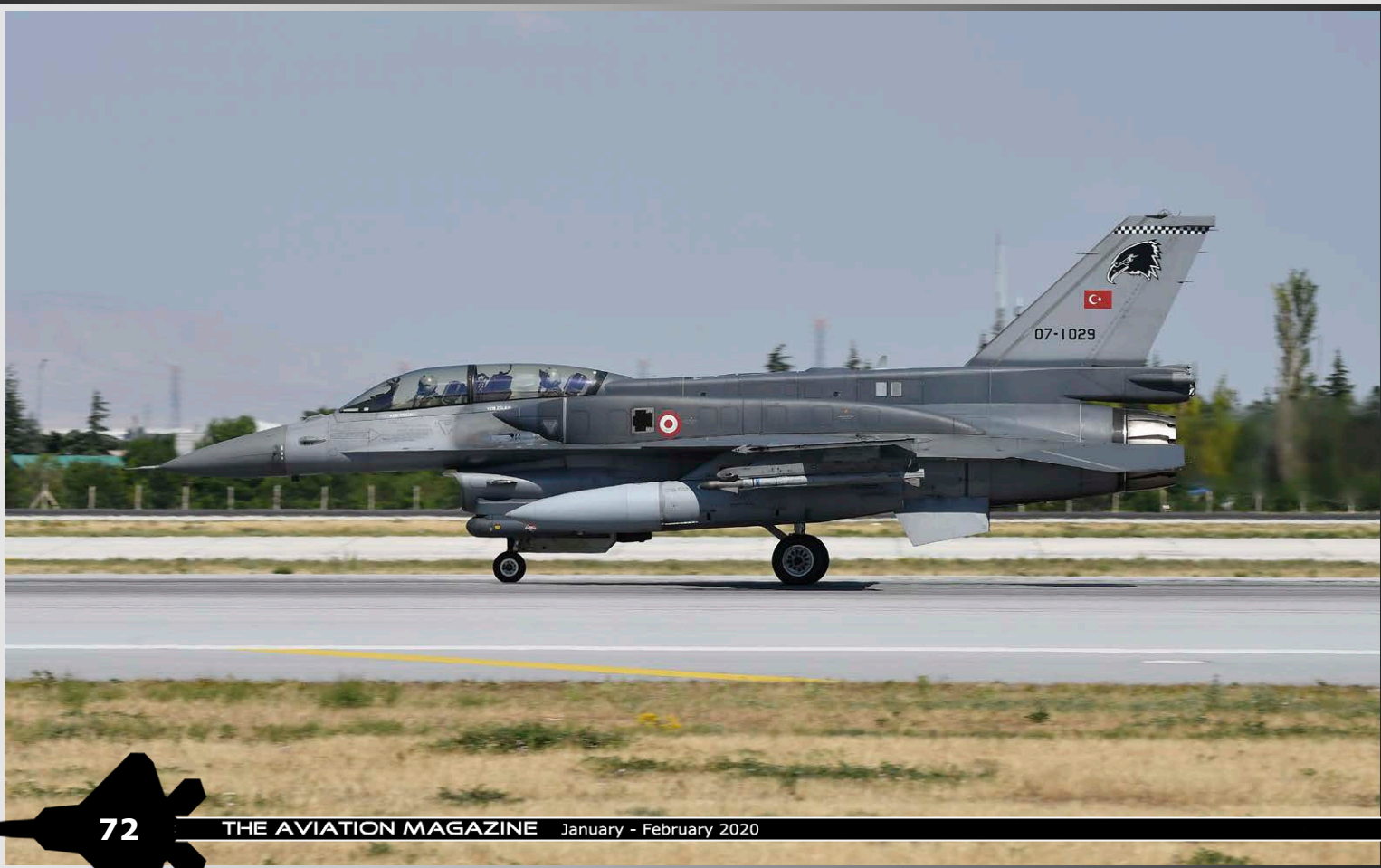
▲ Turkish Air Force F-16D-50+ fitted with conformal fuel tanks, assigned to 161 Filo ▼
