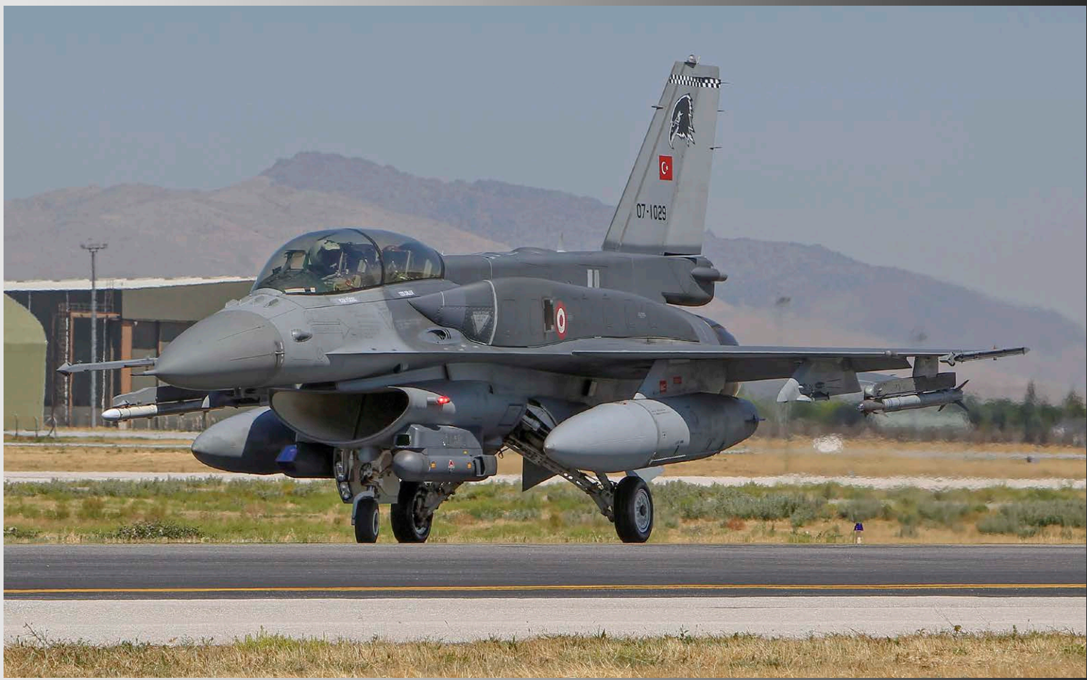
▲ Turkish Air Force F-16D-50+ fitted with conformal fuel tanks, assigned to 161 Filo ▼
