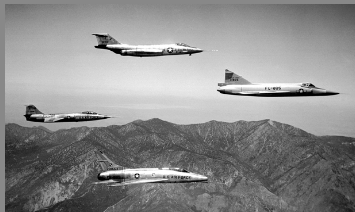
Four century series aircraft in flight. Interceptors were derived from three of the airframes pictured; the McDonnell F-101A-5-MC Voodoo, Lockheed XF-104A Starfighter, and Convair F-102A-20-CO Delta Dagger. Also pictured is a North American F-100A-20-NA Super Sabre. (NACA Dryden Flight Research Center)
