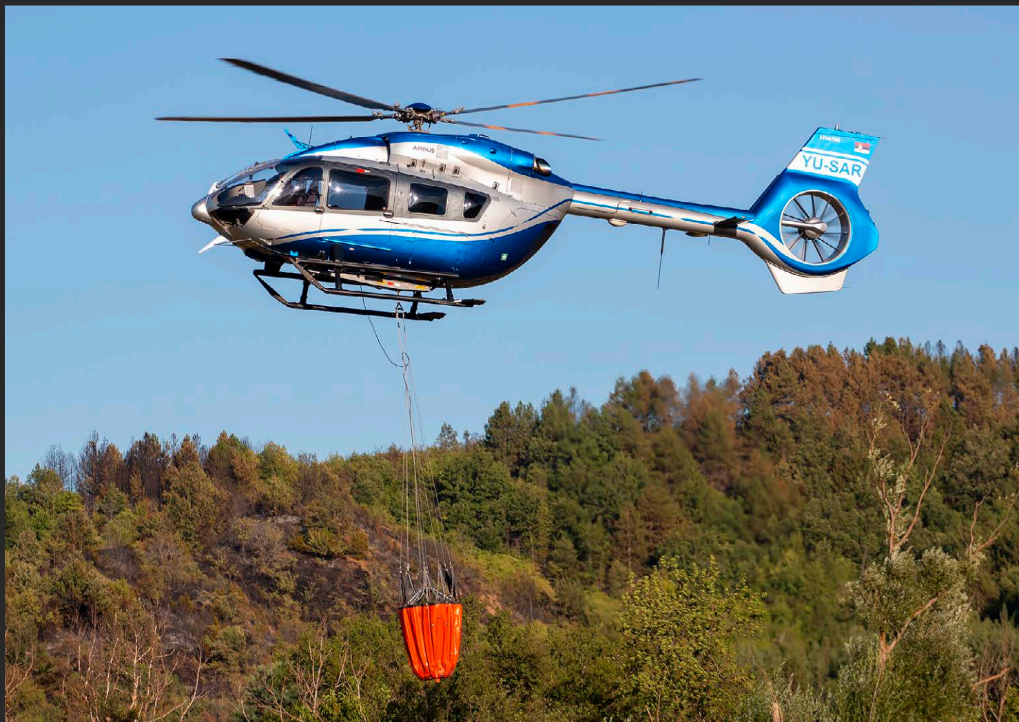
Serbian Police H145M refilling the 800 liter Bambi Bucket with water at Trabotivište. Photo Dragan Cvetic via Igor Bozinovski
