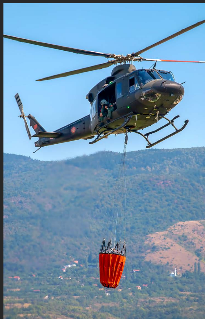
Montenegrin Bell 412EPI XHB033 with 1,600 liters Bambi Bucket. Photo Dragan Cvetic via Igor Bozinovski
