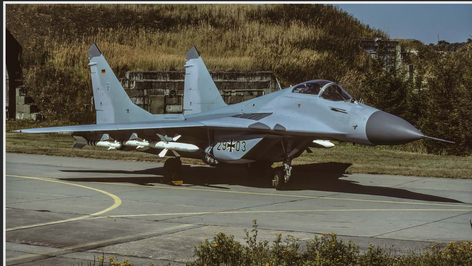
MiG-29G of Jagdgeschwader 73 Steinhoff, ex NVA serial 615 with two R-73E Archer and four R-27R Alamo. Photo Ralf Jahnke ▲ MiG-29A of Erprobungsgeschwader MiG-29, ex NVA serial 670, lost in a crash on 25.06.1996. Photo Ralf Jahnke ▼
