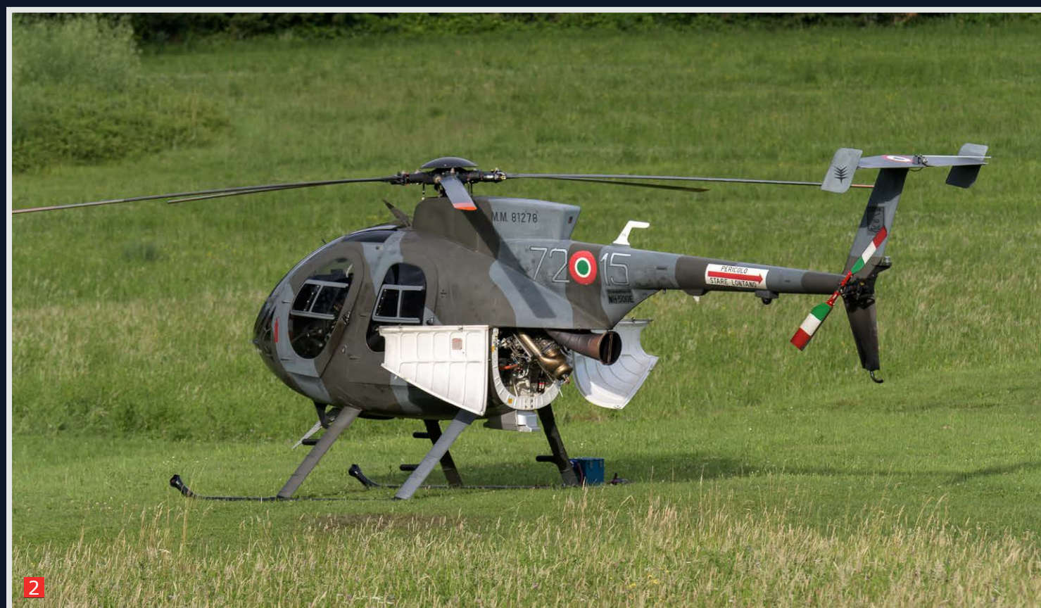
1, 3 The TH-500B is seen at the landing zone while two CNSAS rescue team members are vacating the helicopter. After having dropped off its "passengers", the TH-500B departs the landing zone with guidance from a marshaller. 2 TH-500B parked at its temporary spot in between flights during the exercise with the engine access panels open.
