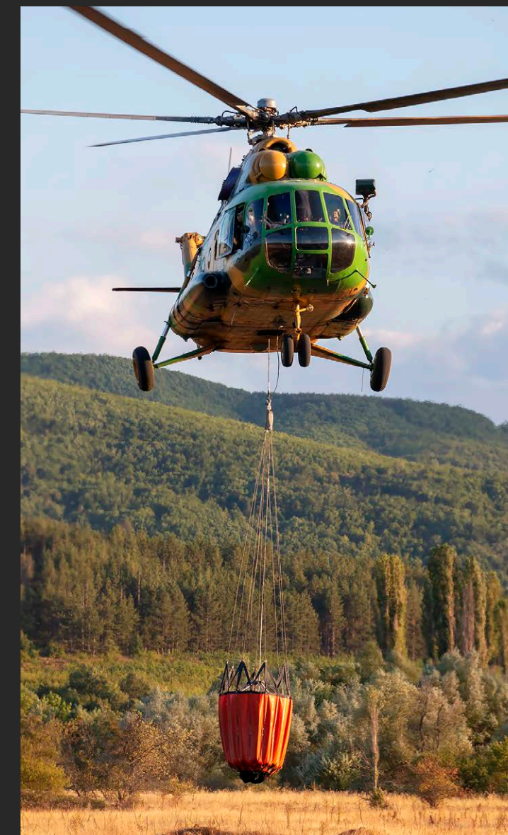
Macedonian AF Mi-17 seen at Trabotiviste with 2,500 liters Bambi Bucket. Photo Dragan Cvetic via Igor Bozinovski
