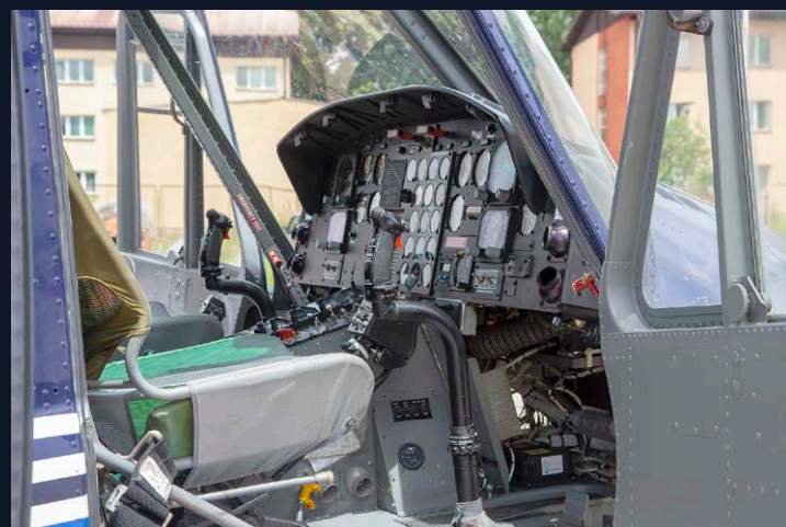
The helicopter now features a modern cockpit instrumentation ( above ). Externally, the FastFin tail boom of the "new" 212 ( top right ) is immediately noticeable compared to the "old" 212 ( top left ).
