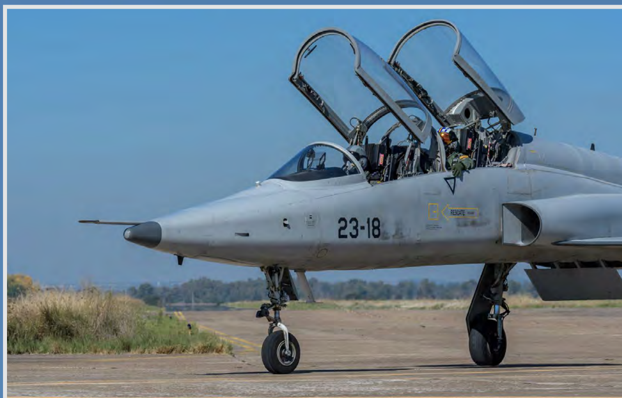
According to the procedures, the canopies of the F-5 should be closed during taxiing. However, the decision to either keep them closed or open both canopies is made by the instructor, depending on environmental conditions. Depicted here is SF-5M AE.9-29/23-18 returning to its parking shed after a training flight.
