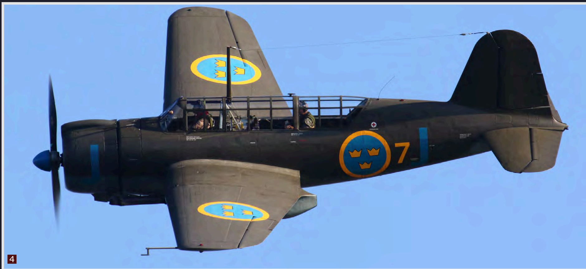
1,2,3 North American SNJ-3 Texan , built in 1942 4,5 SAAB B-17A, delivered to the Swedish Air Force in July 1943. Originally, the B-17 was designed as reconnaissance aircraft. However, it was mainly used as dive-bomber. This aircraft is owned by the Swedish Air Force museum. Its registration is SE-BYH.
