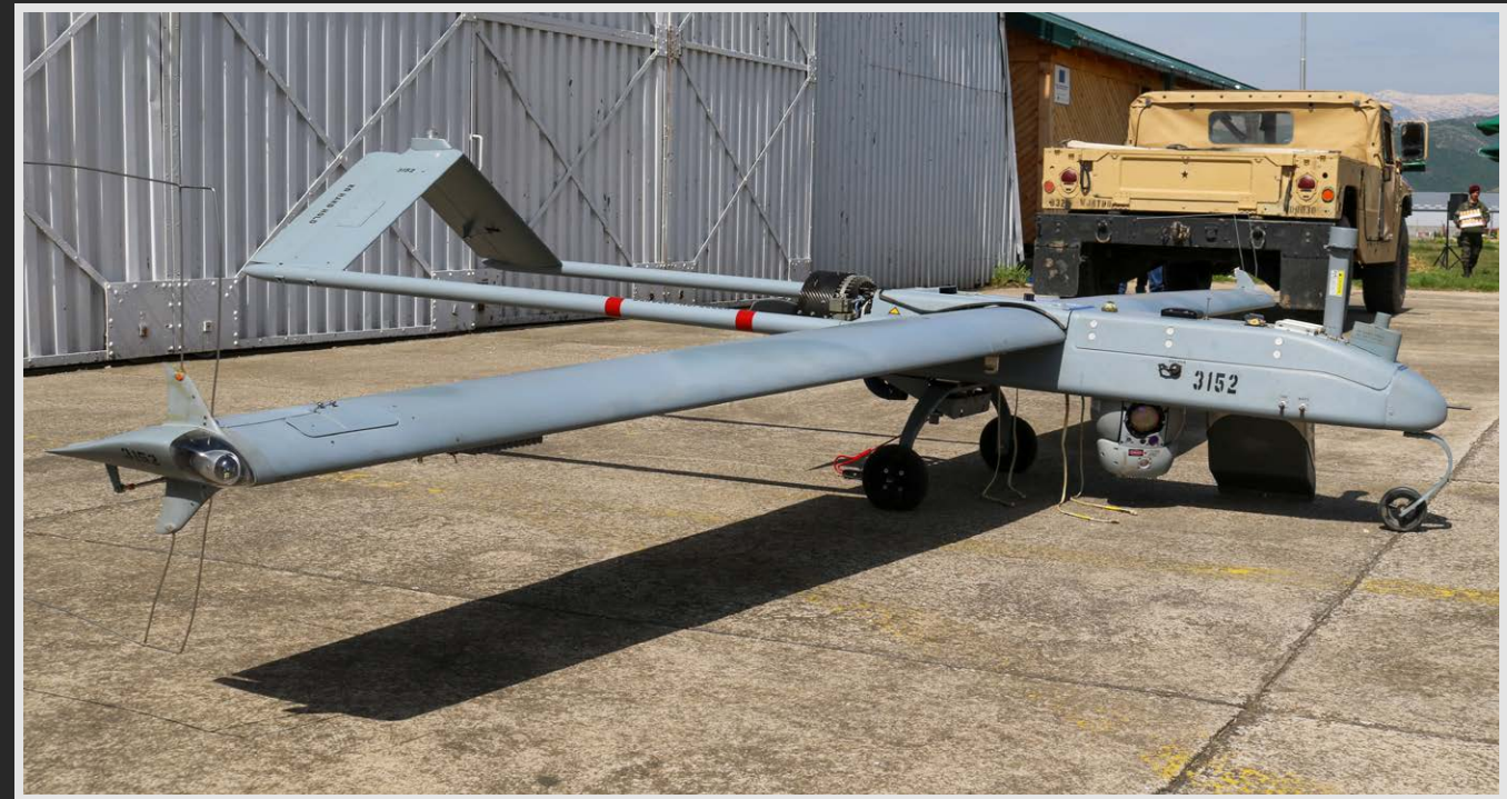
Top: Greece participated in SWIFT RESPONSE with F-16 Fighting Falcons assigned to 330 Squadron based at Nea Aghialos AB. Above: U.S. Army RQ-7 Shadow unmanned aerial vehicle (UAV) used for reconnaissance, surveillance, target acquisition, and battle damage assessment.
