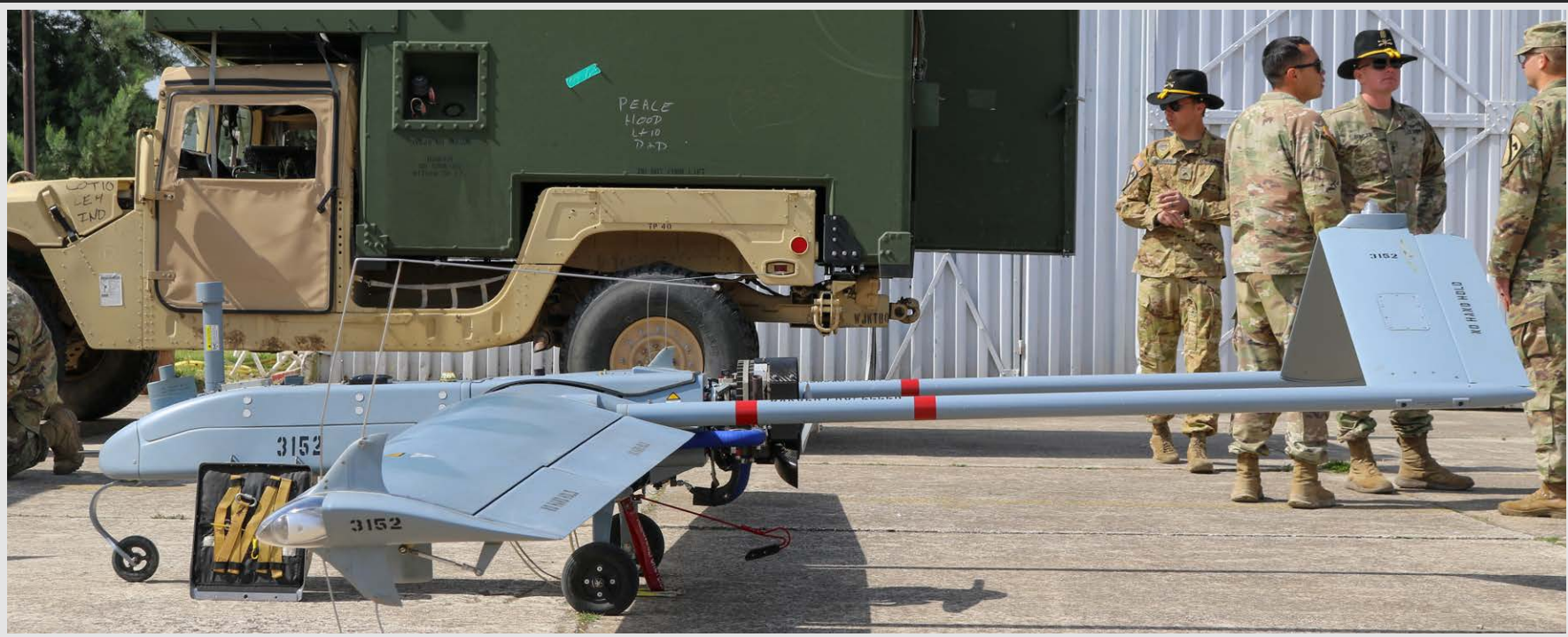
Top: Greece participated in SWIFT RESPONSE with F-16 Fighting Falcons assigned to 330 Squadron based at Nea Aghialos AB. Above: U.S. Army RQ-7 Shadow unmanned aerial vehicle (UAV) used for reconnaissance, surveillance, target acquisition, and battle damage assessment.
